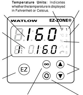
Infinity Key: Press to back up once level, or press and hold for two seconds to return to the Home page. From the Home page can clear alarms and errors if clearable.
