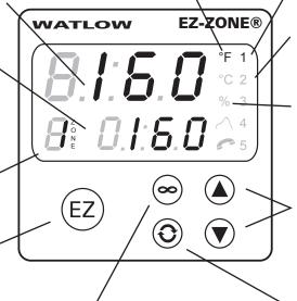
**Infinity Key:** Press to back up once level, or press and hold for two seconds to return to the Home page. From the Home page can clear alarms and errors if clearable. **Output 1 Indicator Light:** When lit it indicates Output 1 is energized.
